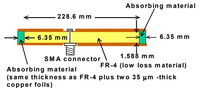
**Figure 3. Cross section of board with absorber (not to scale)**
