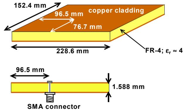
**Figure 2. Experimental structure without absorber (not to scale).**
