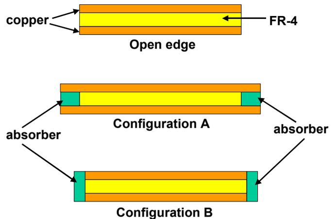
Figure 8. Cross section (not to scale) of open edge board and two methods of mounting the absorbing material.
