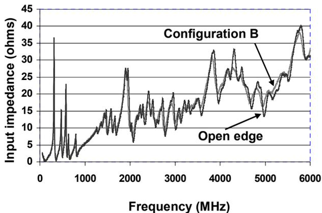
Figure 10. Comparison of input impedance of open edge board with that of board with absorber mounted as in “configuration B” as defined in figure 8. There are only small differences in impedance between these cases.
