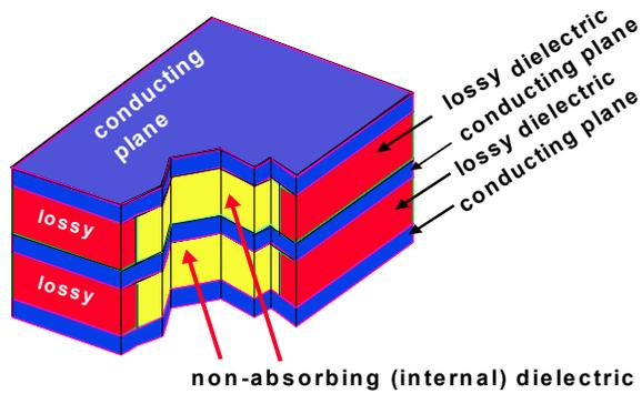
**Figure 1. Basic structure of perimeter-absorber board.**
