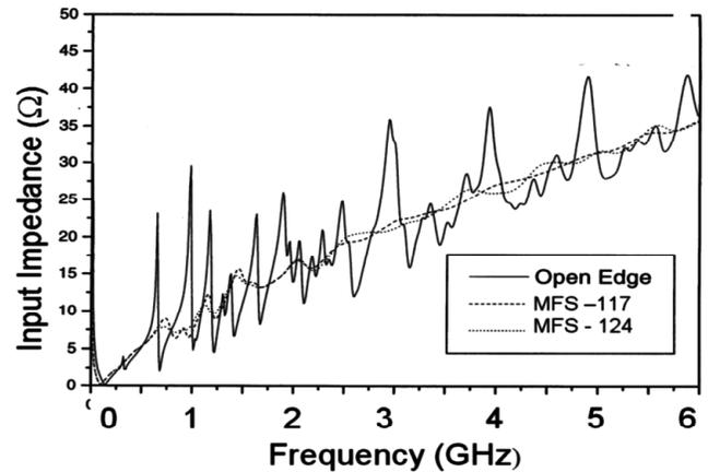
Figure 7. Theoretically calculated input impedance as function of frequency for the three configurations whose measurements are displayed in Figures 5 and 6.
