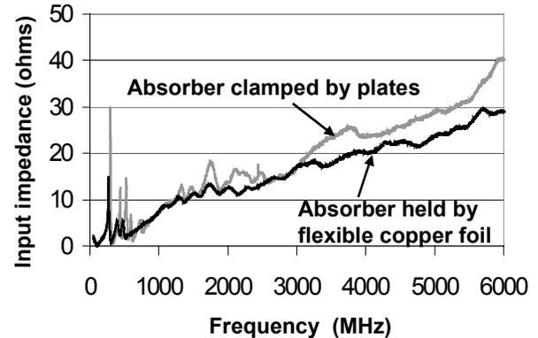
Figure 11. Comparison of input impedance as a function of frequency for absorber clamped between copper plates and absorber held by flexible copper tape.
