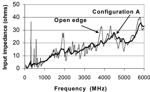
Figure 9. Comparison of input impedance as a function of frequency for open edge board with absorber mounted as shown as “configuration A” as defined in Figure 8.
