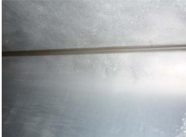
Shown at right as a thin bead of caulking, the ECCOSHIELD VY can fill small gaps left behind during assembly of the aluminum skin. The RF seal created offers in excess of 60 dB over 150 KHz to 10 GHz for electric and magnetic fields and plane waves measured IAW MIL-STD-285.
